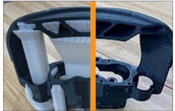
FDM printed Bendix part before and after processing in the PostProcess VORSA 500
