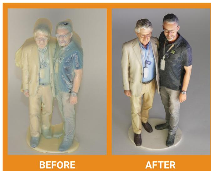
Thanks to integrated software intelligence, users like Marketiger are able to fine-tune the support removal settings to exact parameters, allowing for precise control over the process. The DEMI 400's exclusive additive-formulated detergents, utilized at specified temperatures and in strategized time allotments controlled by the software, ensure consistency and repeatability without part damage or warping.
