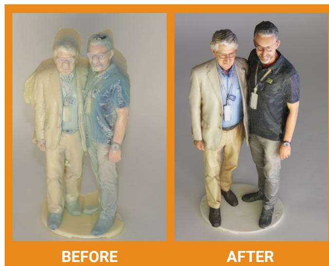
Thanks to integrated software intelligence, users like Marketiger are able to fine-tune the support removal settings to exact parameters, allowing for precise control over the process. The FORTI's exclusive additive-formulated detergents, utilized at specified temperatures and in strategized time allotments controlled by the software, ensure consistency and repeatability without part damage or warping.
