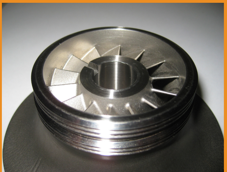
Exacting Surface Finishing of Complex 3D Printed Metal Geometries
