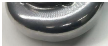
PostProcess Surface Finishing Reveals Intricate Pattern
