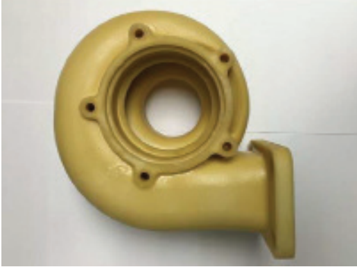
Voxeljet Printer Turbo Casting
