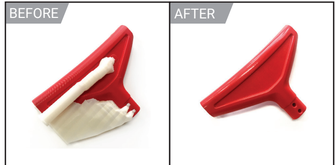
Before: FDM Technology, ABS Build Material, SR30 Support Material
